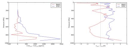
Summary of all comparisons from year 2009. Left: average water vapor differences (IASI-CFH) in ppmv (red) and one standard deviation of the differences (blue). Right: average temperature differences (IASI-SND) in K (red) with one standard deviation (blue) per IASI pressure level.
