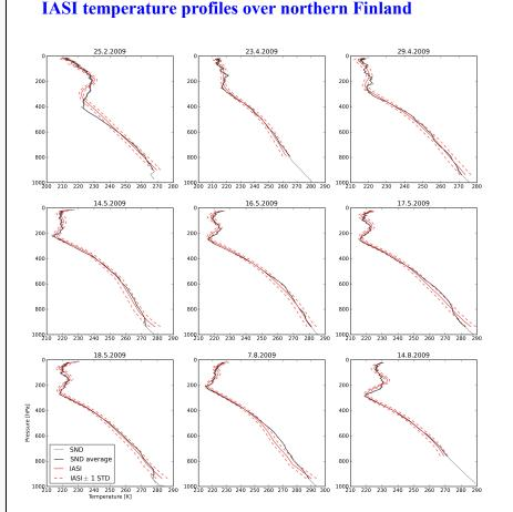
Temperature soundings (grey) and IASI L2 temperature profiles (red) corresponding to the water vapor soundings in figure 2. IASI data is the closest measurement relative to the sonde location at 400 hPa. The dashed red lines indicate one standard deviation of the IASI retrieval. Temperature soundings were averaged to the IASI layers (black solid line).
