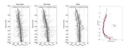
Left: Relative difference between RS92 and the CFH humidity profiles during 7 daytime flights in Sodankyla. The new model is using aluminized coating of the sensor attachment, which reduces the radiation dry bias. Right: CFH/Flash comparison flight on Jan 23, 2009.
