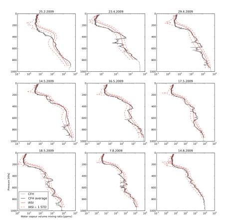
CFH soundings (grey) and IASI L2 water vapor profiles (red) from year 2009. IASI data is the closest measurement relative to the sonde location at 400 hPa. The dashed red lines indicate one standard deviation of the IASI retrieval. CFH soundings were averaged to the IASI layers and all comparisons were made between the CFH average (black solid line) and the corresponding IASI value.
