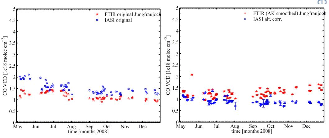
As expected from the averaging kernels we see an increase of the FTIR CO total columns after the smoothing. Also expected for the mountain site Jungfraujoch (3580 masl) when the IASI total columns are corrected to the altitude of the gb FTIR site, the columns decrease. The altitude correction is done using the TM4 model by calculating a correction factor based on the ratio of the total column over the g-b site's altitude to the total column over the IASI pixel altitude.
