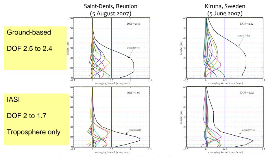
The colored horizontal dashed lines indicate the height for which the corresponding colored kernel is active. The sum of the rows of the averaging kernels is indicated in black. The numbers of degrees of freedom for signal (DOF) are shown in the plots
