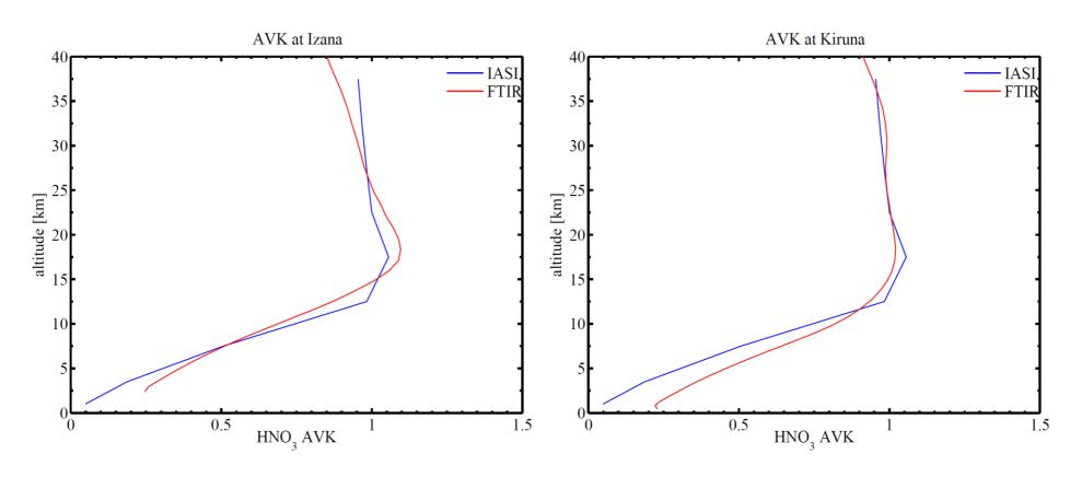
The total column sensitivities are similar for the HNO3 retrievals from ground-based solar absorption spectra and from IASI radiances. They show that the retrievals are most sensitive in the stratosphere. This means that tropospheric HNO3 has a minor influence on total column HNO3, and topographical differences have only secondary influence on the total column.
