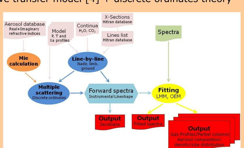
• This code offers the possibility to retrieve vertical concentration of atmospheric constituents (gas, liquid, solid) simultaneously from spectra, which may have been recorded by different instruments (from IR to UV).
