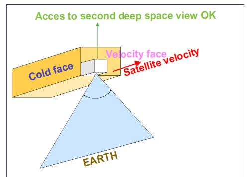
IRS accomodation on the satellite velocity face
