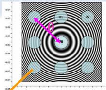
IASI-NG: Optical signal in the detectors plane for v=2760cm-1 and OPDmax=4cm
