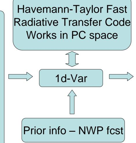
Output profiles of: •Temp(z) •Wat Vap (z) •Ozone (z) •Surf Temp T\* •15 Emissivity PC scores
