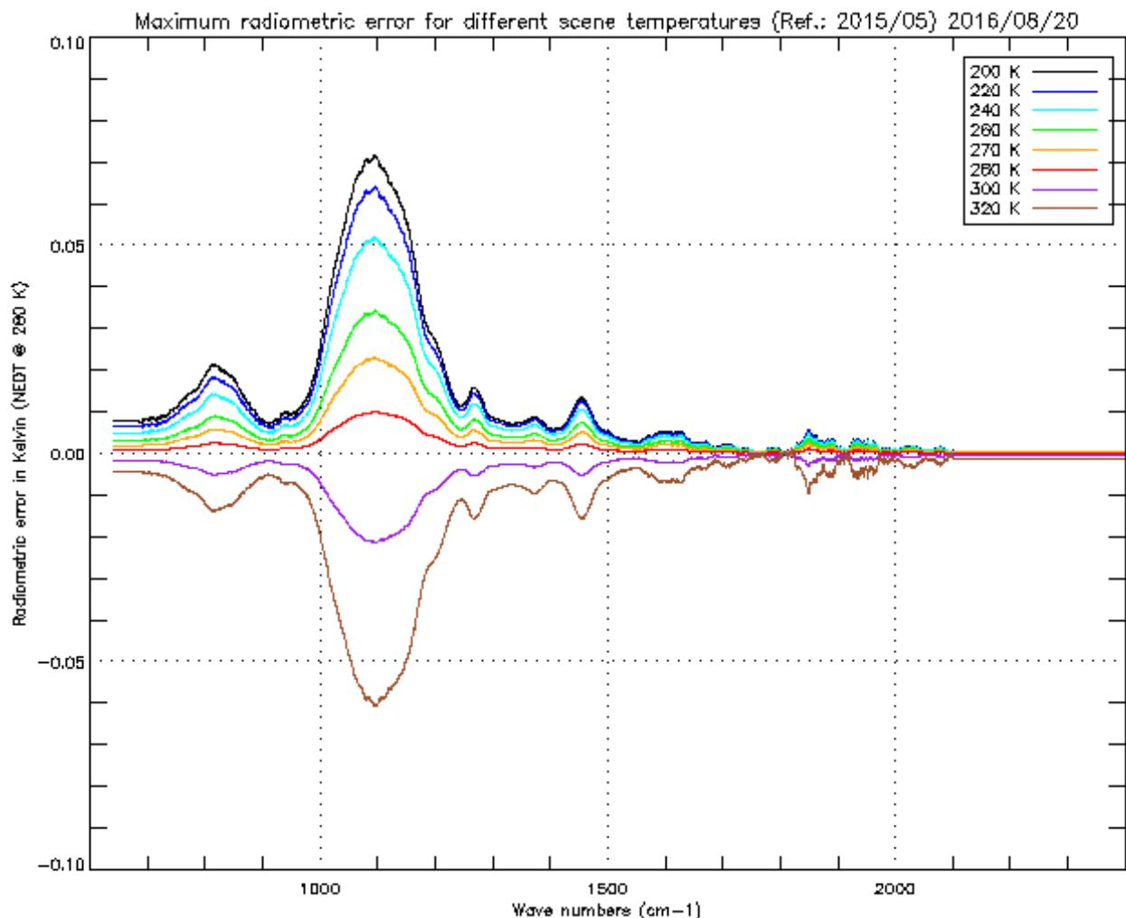
*Figure 23 : Radiometric calibration error due to scan mirror reflectivity dependency with viewing angle Maximum effect on SNI for different scene temperature.
