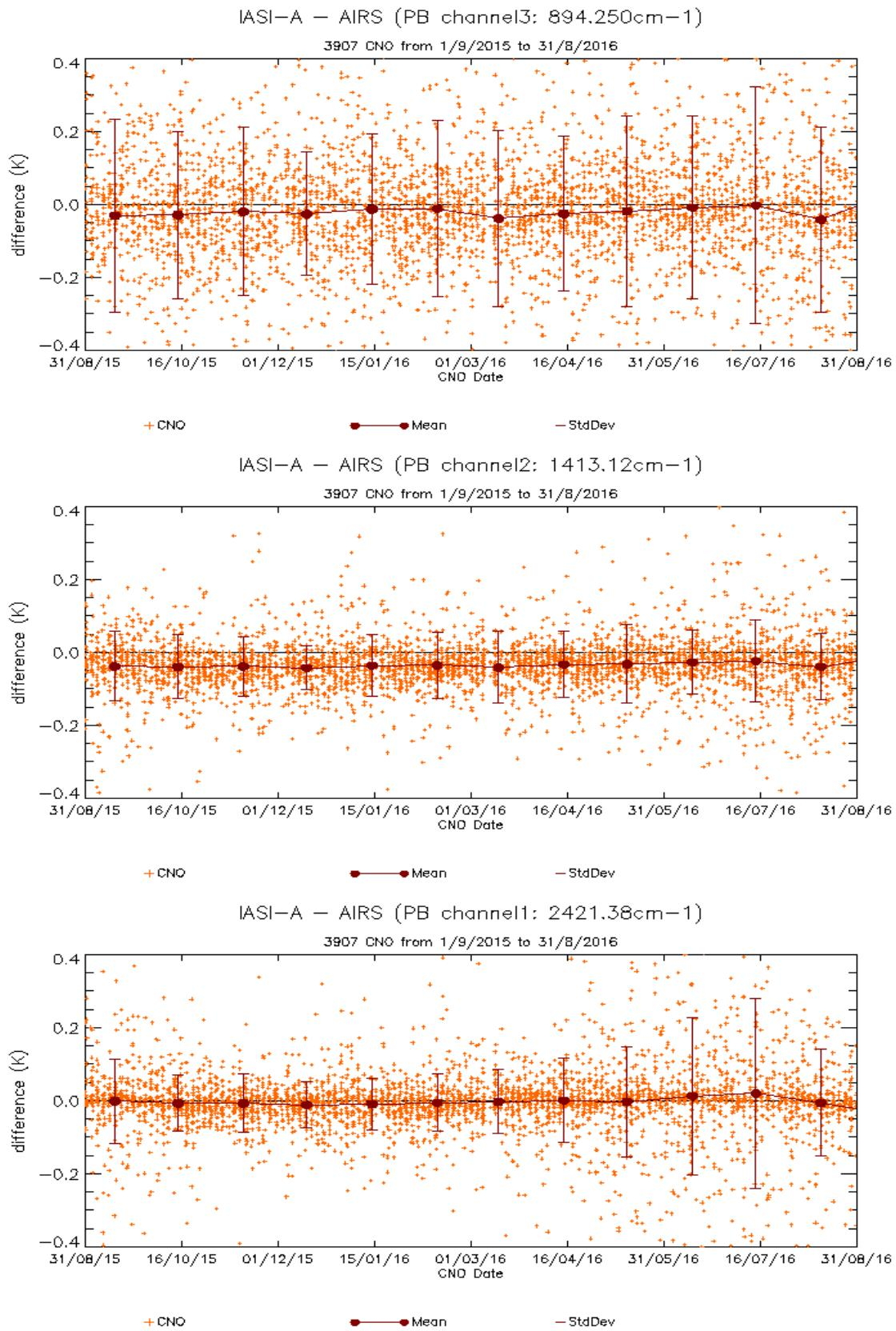
Figure 41 : Temporal evolution of the differences IASI-A – AIRS in brightness temperature over the approximate three IASI bands, with monthly means
