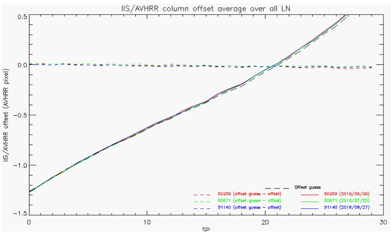
*Figure 36 : Column offset (black) guess vs. column offset averaged over all lines (LN)
