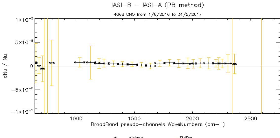
*Figure 40 : Mean (black curve) and standard deviation (yellow curve) of the difference spectral calibration  $\Delta v/v$  between IASI-B and A.*
