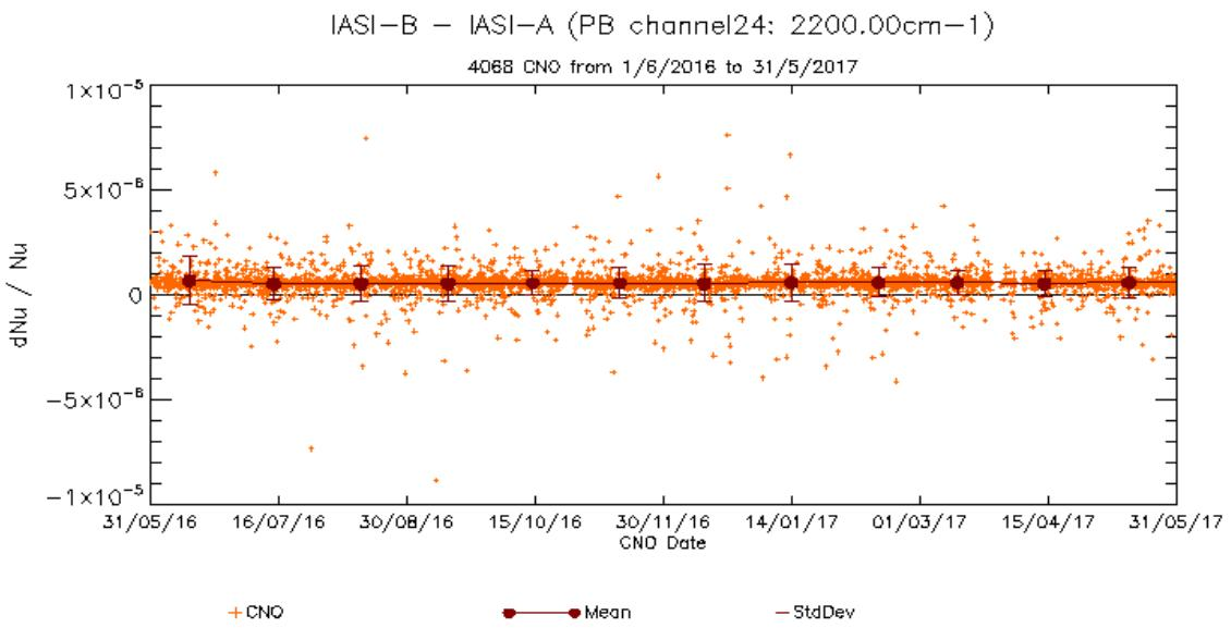
*Figure 41 : Temporal evolution of the difference spectral calibration  $\Delta v/v$  between IASI-B and A in the spectral window centered around 2200 $\text{cm}^{-1}$ .*
