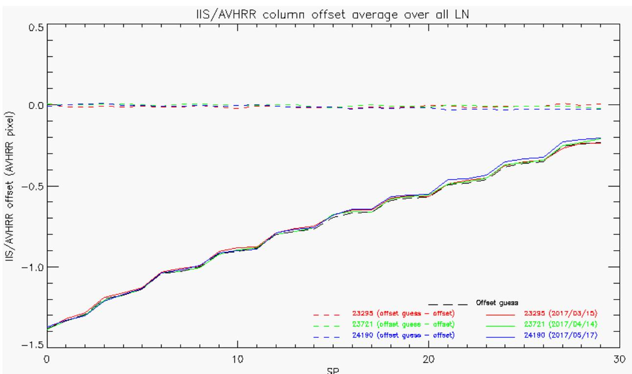
*Figure 36 : Column offset (black) guess vs. column offset averaged over all lines (LN) as a function of the scan position (SP=SN), and orbit number*
