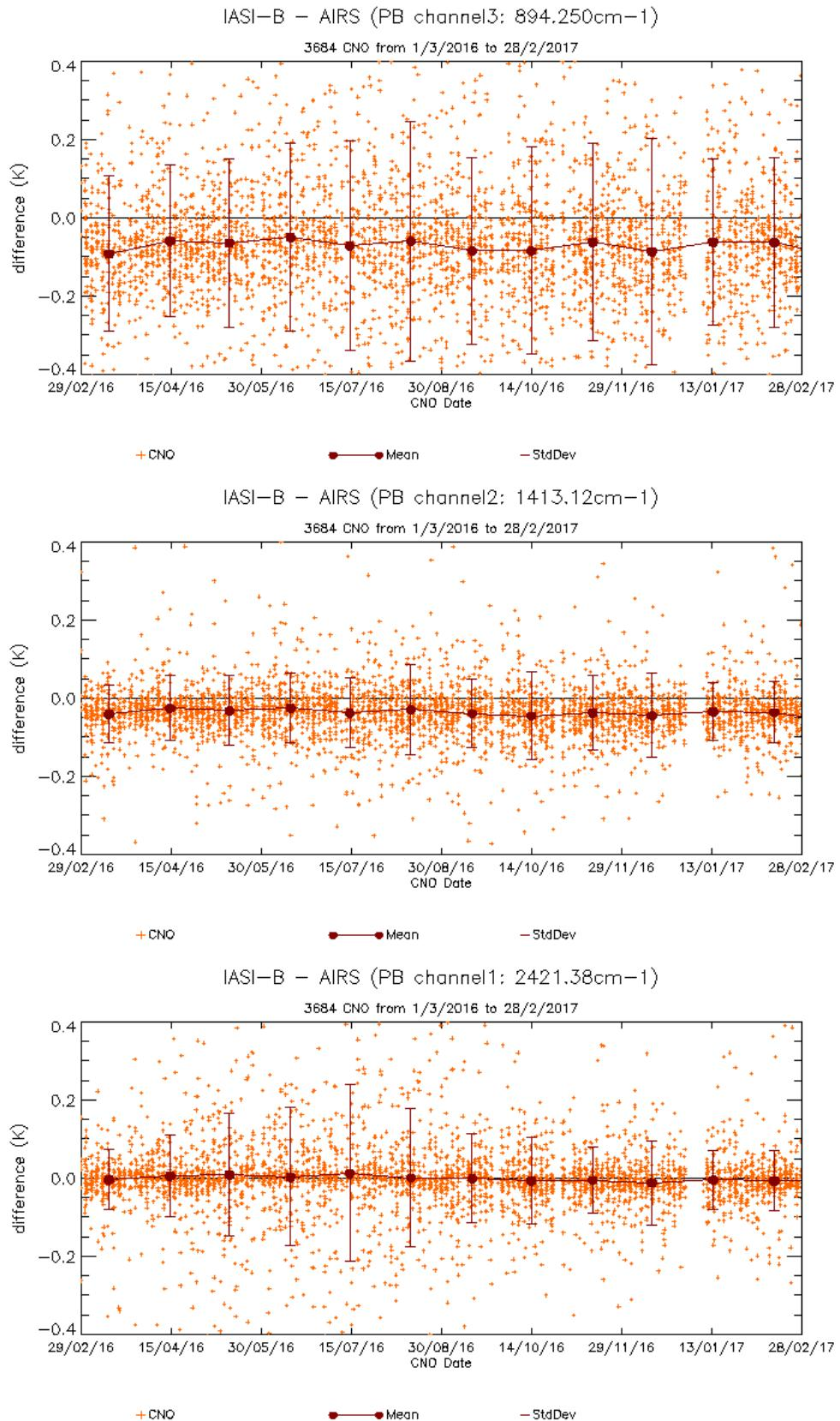
*Figure 45 : Temporal evolution of the differences IASI-B – AIRS in brightness temperature over the approximate three IASI bands, with monthly mean.*
