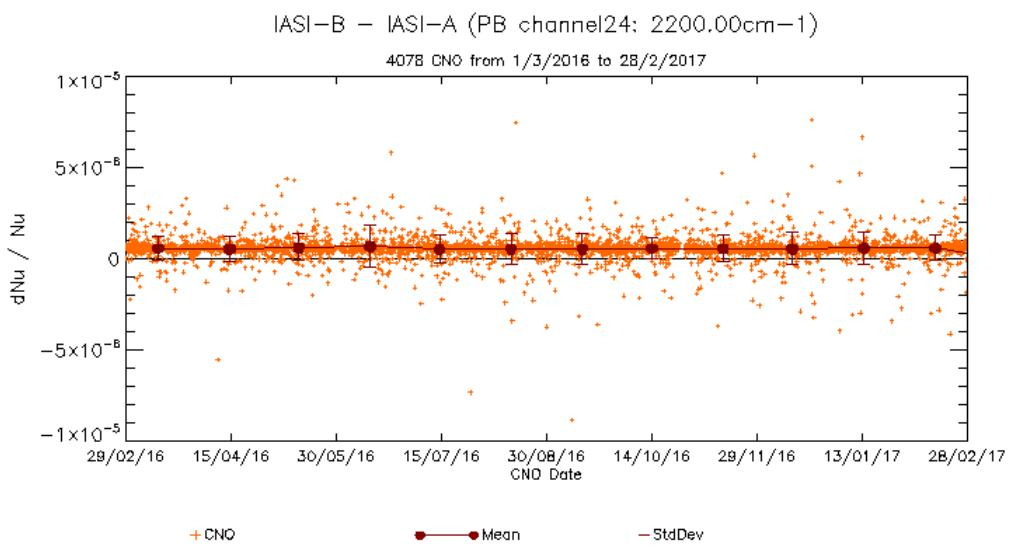
Figure 41 : Temporal evolution of the difference spectral calibration  $\Delta v/v$  between IASI-B and A in the spectral window centered around 2200cm $^{-1}$ .
