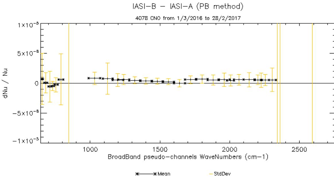
Figure 40 : Mean (black curve) and standard deviation (yellow curve) of the difference spectral calibration  $\Delta v/v$  between IASI-B and A.
