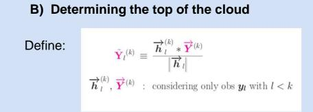
if for all levels *l*:  $\tilde{\mathbf{Y}}_{I}^{(k)}$  < Threshold 1 is designed to filter (mainly) cloud type structures  $\operatorname{grad}_{k}\left[\tilde{\mathbf{Y}}_{l}^{(k)}\right] < \operatorname{Threshold} 2$ Flag FoVs cloudy where Y exceeds threshold
