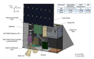
CIRAS, the codename for the prototype of the 5um sounder, meets the requirements of the 5um sounder and fits into a 6 liter (6U in CUBESAT terminology) package, compared to the 800 liter envelope of CrIs. This volume difference alone results in a more than one order of magnitude cost decrease. This makes CIRAS a candidate for deployment on a CUBESAT constellation. The first CIRAS is currently funded by NASA for launch into polar orbit in late 2019.
