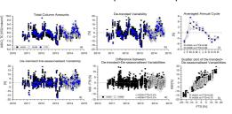
Example for the decomposition of O3 time serie in measurement-to measurement and annual cycle (in blue circles FTS, in black squares IASI-A and in white circles IASI-B)
